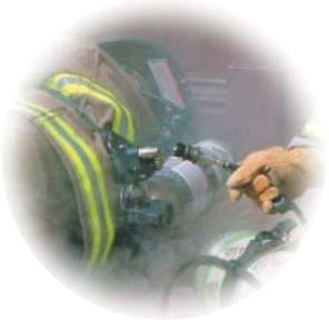
The Quick-Fill<sup>®</sup> URC is a universal rescue connection located within 4" of the cylinder valve outlet in the Audi-Larm™ housing.
